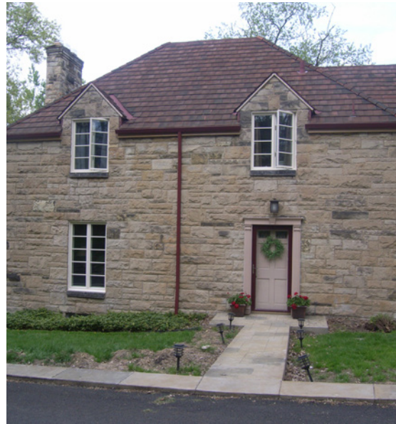
Hipped Roof common on French Provincial, Craftsman, Foursquare and Colonial Revivals
